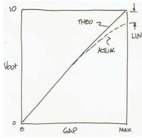
Uncorrected linearity can be 2-5%. One source of nonlinearity is the non-zero input capacitance looking into the cable. As the sensor capacitance can be ~0.1pF, for uncorrected 1% linearity the input capacitance must be <0.0001pF.
