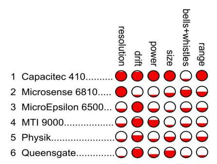
The comparison results (detail below) rank Capacitec #1, with solid performance in the most critical parameters, best range, and excellent stability with different cable lengths. Microsense takes the resolution award, and Micro Epsilon the drift award. Physik has an accurate probe assortment.
