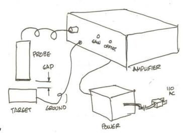
The amplifier accepts a coax or triax cable to the sensor, with often a fixed 1m cable length. Some manufacturers allow extension cables to 10m without recalibration. Shorter cables are less noisy due to the lower signal-to-guard capacitance. Some manufacturers offer active probes, or an active preamp in the cable, for long cable runs but limited temperature range.
